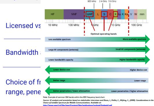
Frequency diagram sourced from Southwest Antennas, Inc. (2016). Modern Co-Site RF Interference Issues and Mitigation Techniques. Based on "Frequency Band Comparison" by Treinkvist. Please see: <u>https://southwestantennas.com/sites/default/files/white-</u> poper/Whitepaper. Modern-Co-Site-Interference-Mitigation-Techniques. Southwest-Antennas.pdf
